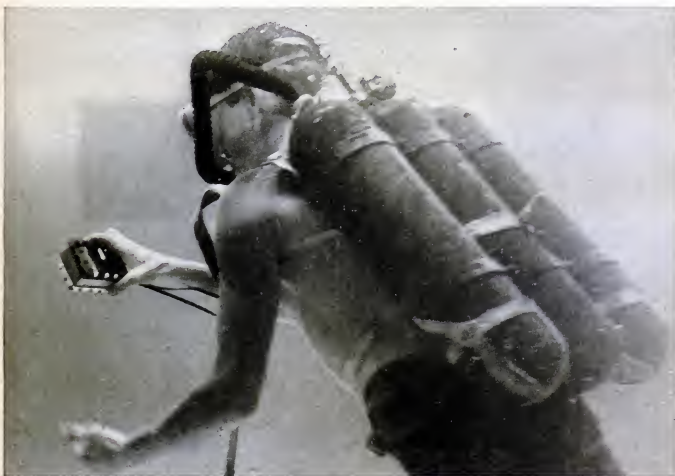
Underwater cameraman uses an exposure meter made waterproof with a metal-plastic case.
